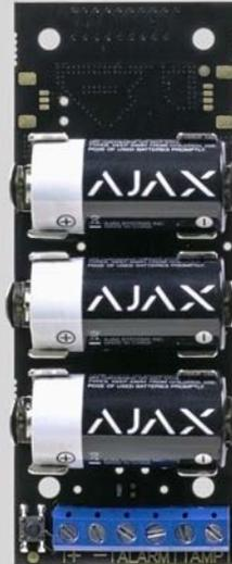
**Transmitter** is a module for connecting third-party detectors to Ajax security system. It transmits alarms and notifies when the tamper of the third-party detector triggers. The module is equipped with its own accelerometer, which protects it from dismounting. It runs on batteries and can supply power to the connected detector.
