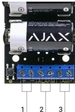
1. “+ -” – power terminals of the connected wired device, the output voltage is 3.3 V<sub>DC</sub>.
